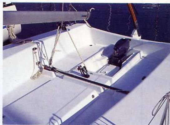
Left, control lines are all led aft. Above, the outboard well lid is securely held forward of the mainsheet traveller when the engine is in use
